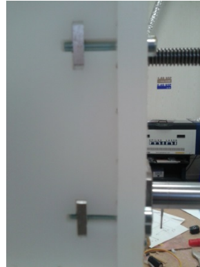
Figure 3: (Left) Original “Snap” junction; (Right) Re-designed bolt interface with metal nut-plate
