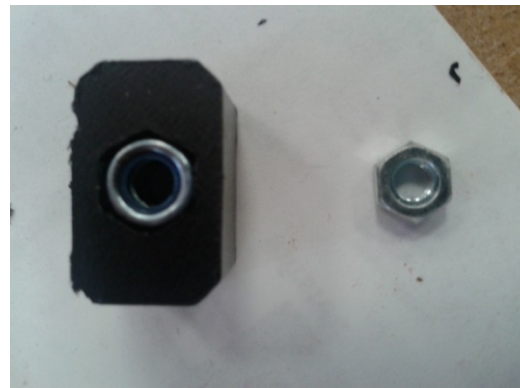
Figure 4: (Left) Re-designed bolt interface with plastic “nut-adapter” installed; (Right) “Nut adapter” shown exposed with M5 nut
