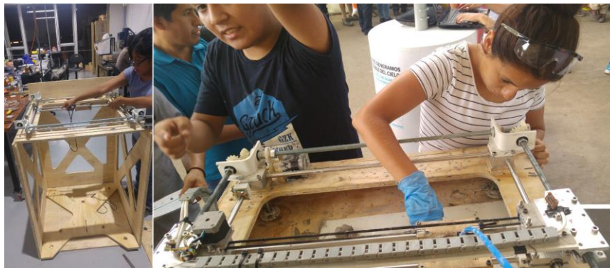
Figure 13: large format clay 3D printer developed during the summer.
