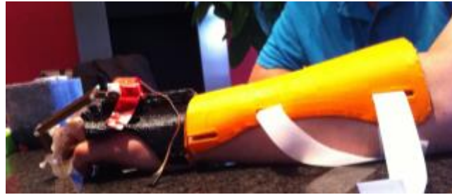
Figure 16. Testing the part and the interaction of the Myoware connection of the Myoware to the SatshaKit and assembling the Satshakit + Myoware + Motor + Orthotics Prototype. https://youtu.be/kyQ4P8TT0I
