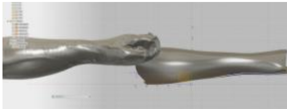
Figure 4. Free Form in 360 function from Fusion 360 software allowing the creation of mesh nodes in X and Y direction which are attached in the original 3D Scan.
