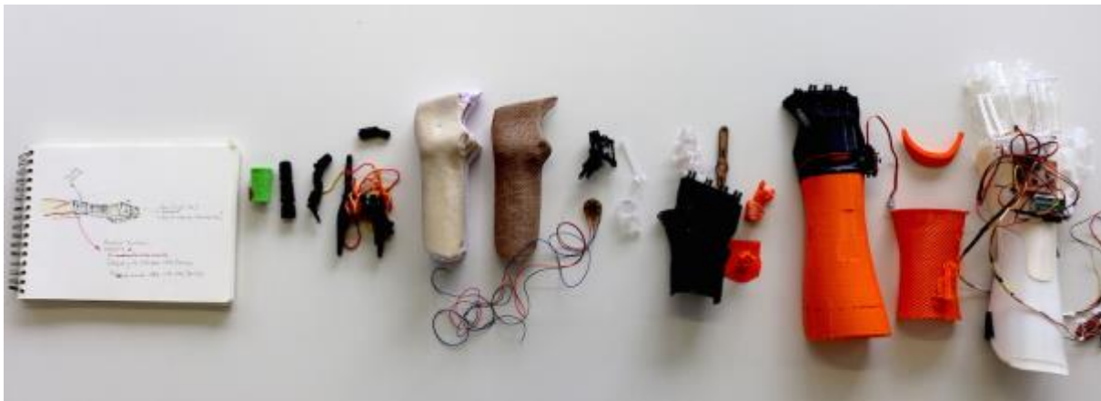
Figure 1: Development from the sketch to the final prototype using traditional and digital prototyping technique to produce MyOrthotics.
