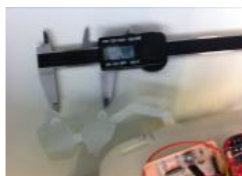
Figure 15. 3D Printed Thumb phalanges testing the accuracy and calculating the size of the exoskeleton connections.
