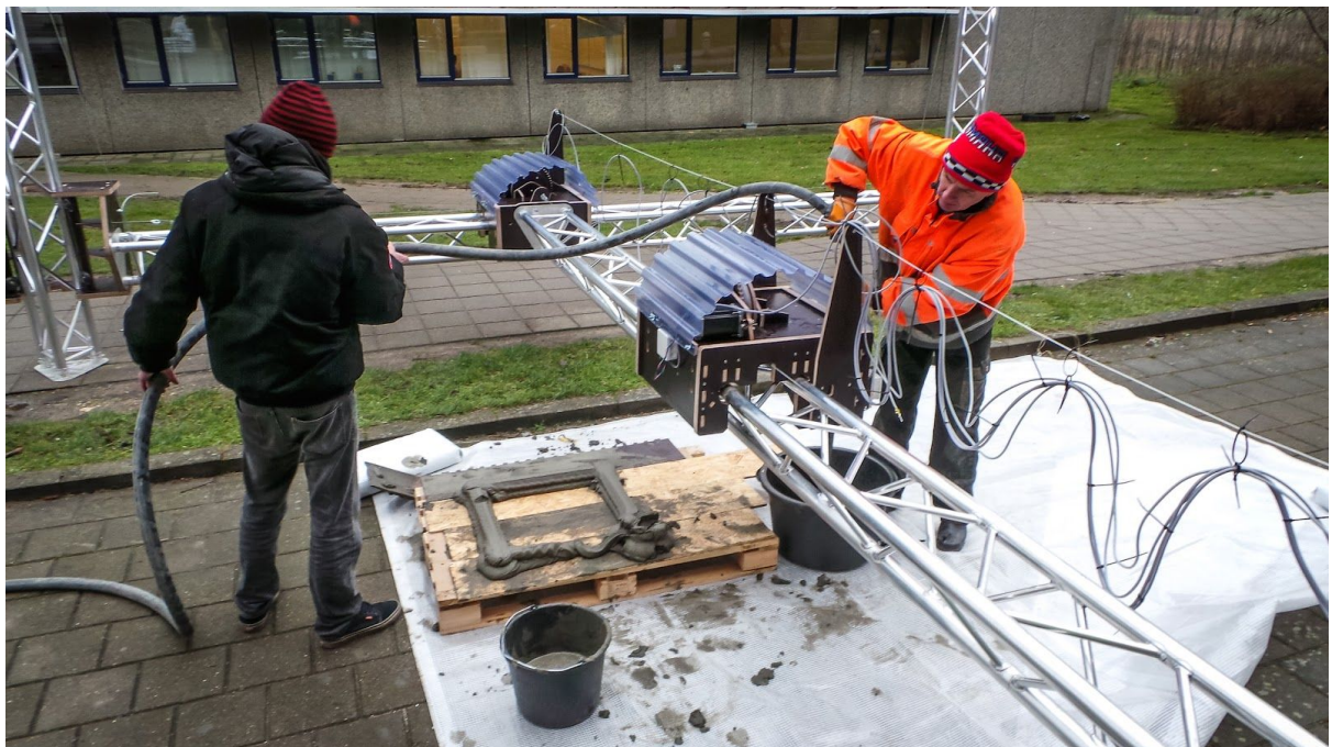
Figure 2: First experiments with the 3D printer printing concrete.
