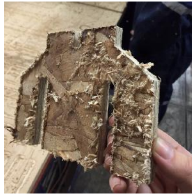
Figure 5: A piece of the junction, made with 10mm recycled wood board.
