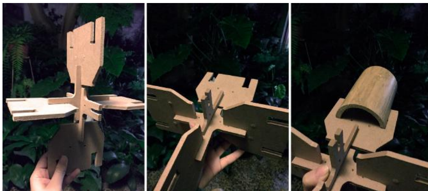
Figure 8: Junction made with 6mm MDF board.
